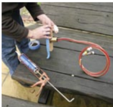
The keel cooler was carefully masked around its outer edges to protect them from excess sealant. Any sealant stuck here will act as an insulator, reducing the unit's efficiency
